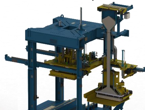
closed filling-system for shoot unit in inorganic production - no sand dry out -
